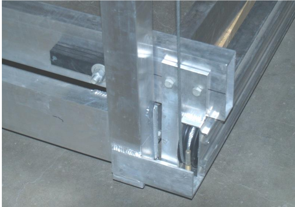
Cable comes over pulley and DOWN to angle bracket or under pulley and UP.
