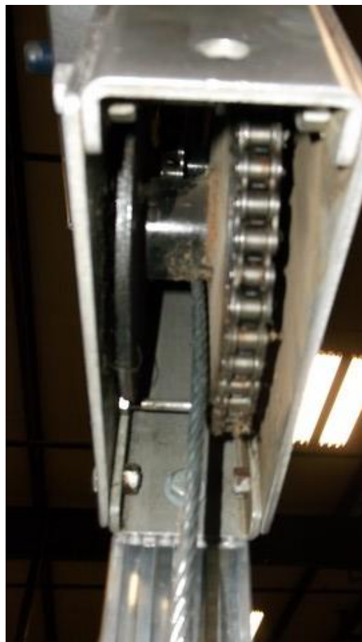
Cable inserted into Drum center hole
