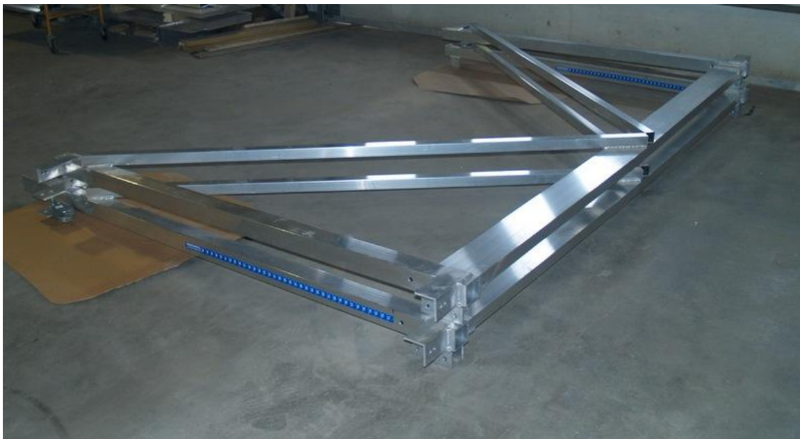
Left and right side welded assemblies.
