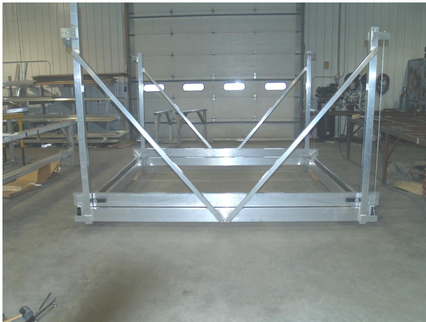
Assembled boatlift frame with cross members bolted in.
